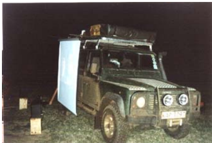
When a building or tree is not available, the screen is hung from the roof of the rover
